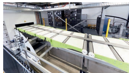
The strip is transferred to the downstream press or punching machine via a loop pit with a radius of 2,000 mm. If required, the strip can be transferred horizontally via a strip transfer table.
