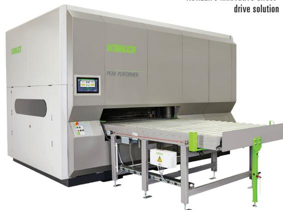
KOHLER Peak Performer, a hydraulic-free part levelling machine
