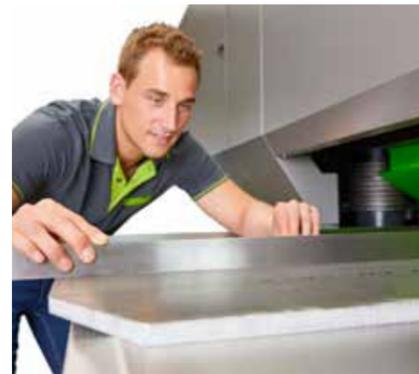
— The Peak Performer part levelling machine also levels thick sheets with great precision
