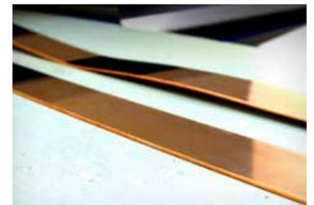
— The levelling result achieved by the Peak Performer 50P.600 is clear; at the top you see the (gold) strip prior to levelling, and below is the levelled, even, absolutely flat strip.
